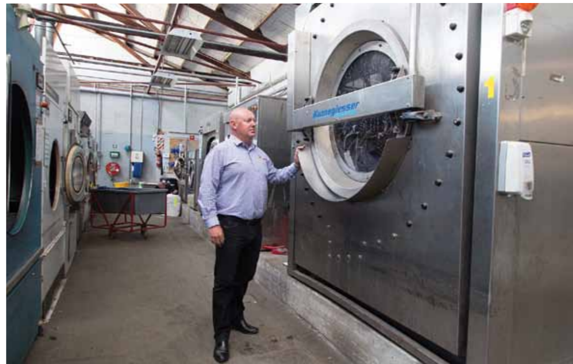
Bevan Ritchie shows off the huge washing machine that can work through 195kg of garments per cycle.
